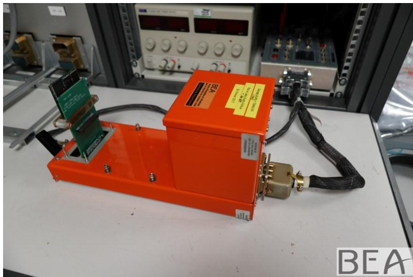
Figure 38- CVR memory card read-out at BEA laboratory using donor-chassis- Photo: BEA
