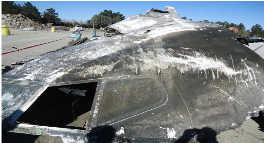
Figure 14 - Closer view of the cockpit
