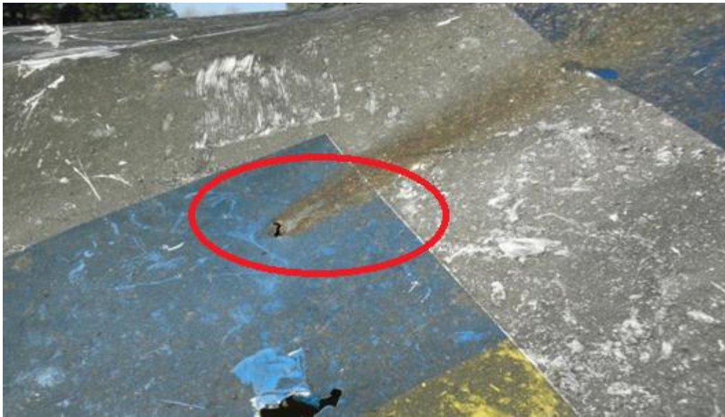
Figure 16- Hole in the fuselage with a trace of a different color of smoke
