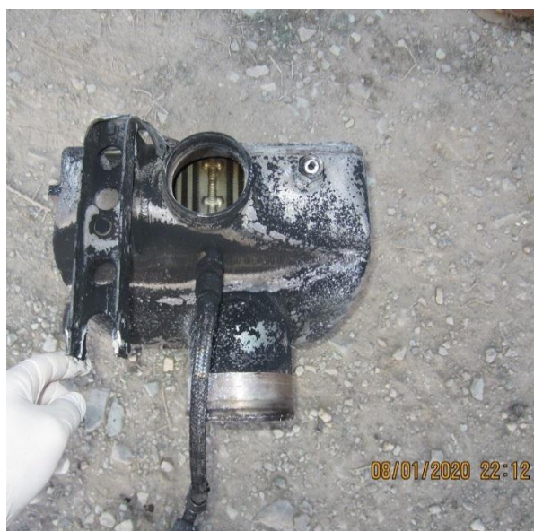
Figure 10- A part of air conditioner found on ground before crash site
