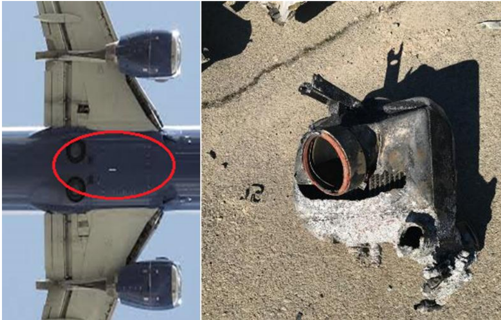
Figure 22- The second heat exchanger found at the accident site and its installation point on the fuselage
