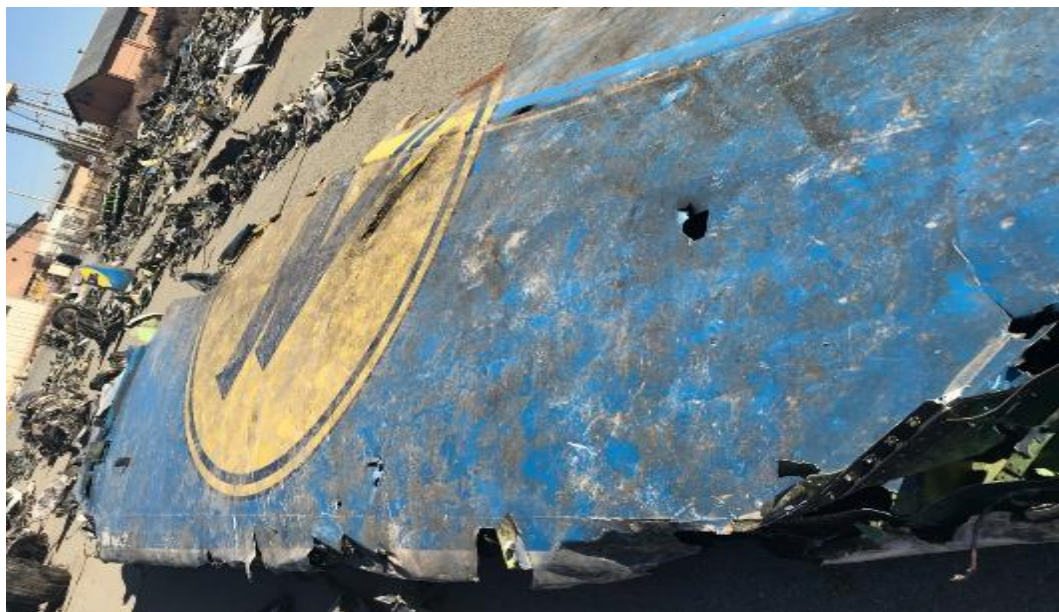
Figure 21- Holes and cracks on vertical stabilizer
