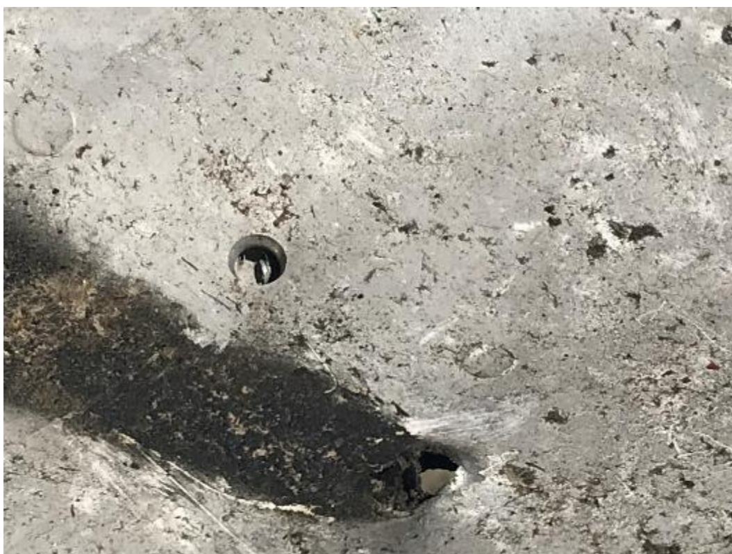
Figure 19- Closer view of the hole on the fuselage near the cockpit and burn signs in the hole area
